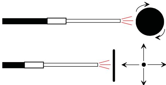
With **REFLECTANCE COMPENSATED Sensors**, the output voltage is only proportional to the distance between the sensor tip and the target surface.
