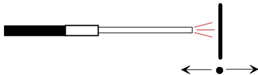
With **REFLECTANCE DEPENDENT Sensors**, the output voltage is proportional to the distance between the sensor tip and target surface **AS WELL AS** the reflectivity of the target surface.
