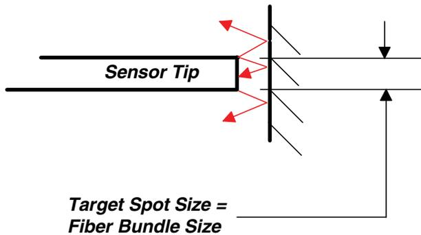
Any light rays diverging outward and away from the perimeter of the sensor tip are reflected further away from the tip. Therefore, **the target spot size is equal to the area of the fiber- optic bundle in the sensor tip**. The target should be equal to or larger than the fiberoptic area to achieve rated specifications.
