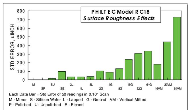
NOTE. The Surface Roughness Standards used in these tests are calibrated in microinch AA with contact gaging. The total Peak-to-Valley depth of Roughness...which is the profile "seen" by the RC18 fiberoptic sensor...varies from 4 to 12 times the AA values. This difference between contact and non-contact gaging can explain why the fiberoptic data does not match the contact gage data 1 to 1 throughout the range of specimens.
